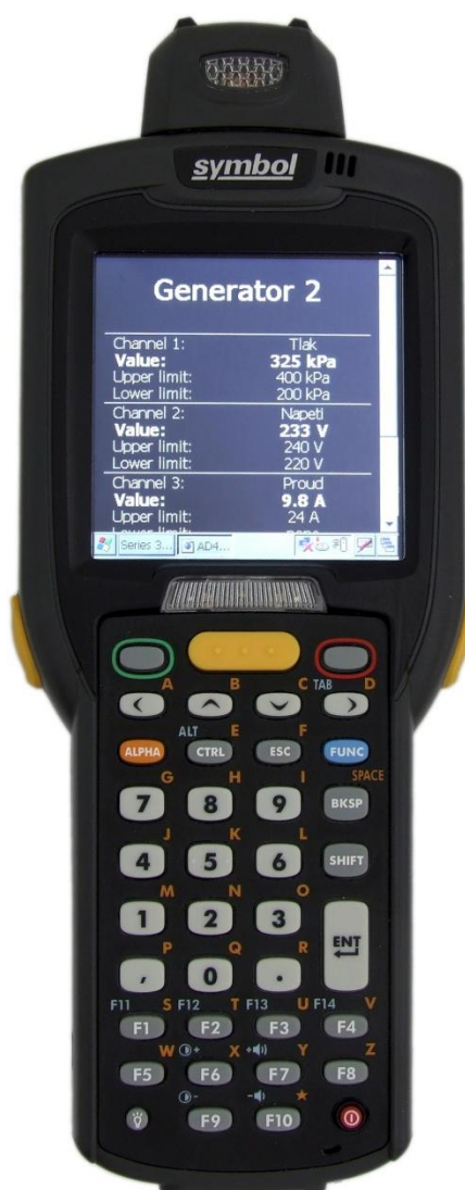
Fig. 9 – Example of WAP interface opened in a mobile device
