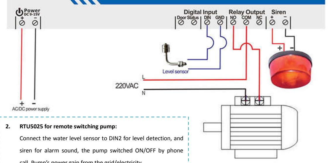
**2. RTU5025 for remote switching pump:**
