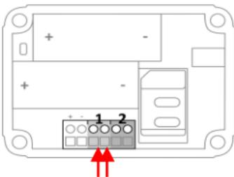
As default the inputs are programmed as Normally Open (NO) contacts. This means the inputs are triggered if the input is closed for at least 1 second. In case the contact is Normally Closed (NC), please refer to paragraph 5.6. If you require the sensor to be activated for a shorter or longer period before triggering an alarm, please refer to 5.6.
