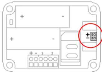
**NOTE:** The output does not work if the CML2255 is battery-operated.
